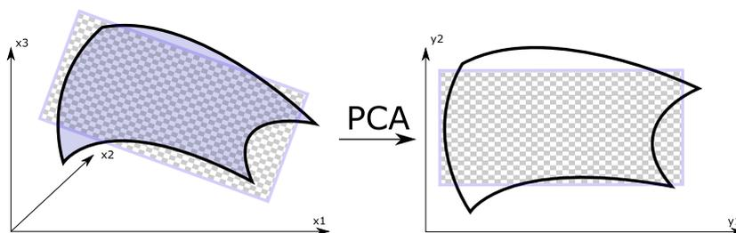
Figure 5: An embedding of a manifold in two-dimensional Euclidean space, using Principal Component Analysis. The manifold on the left is already embedded into three-dimensional Euclidean space, but PCA is able to find a two-dimensional embedding, because the manifold is almost planar.
